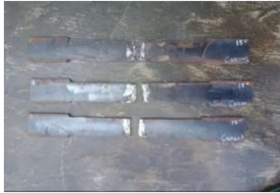
Gambar 2. Hasil pengujian Speciment media pendingin collant 15°C
