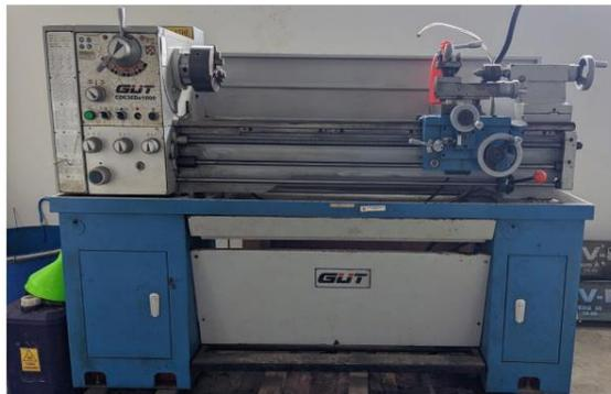
Gambar 4. Mesin bubut GUT C0636D X 1000 di laboratorium terpadu ITK
