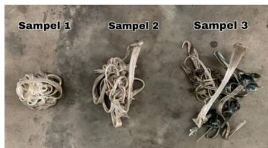
**Gambar 7.** Hasil lelehan *styrofoam* temperatur 240-250 °C
