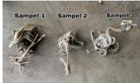
**Gambar 6.** Hasil lelehan *Styrofoam* temperatur 220-240 °C
