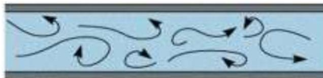
Gambar 2. Pola garis arus aliran turbulen
