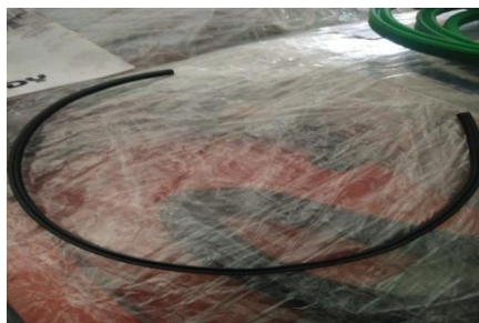
Gambar 12. Seal piston rusak
