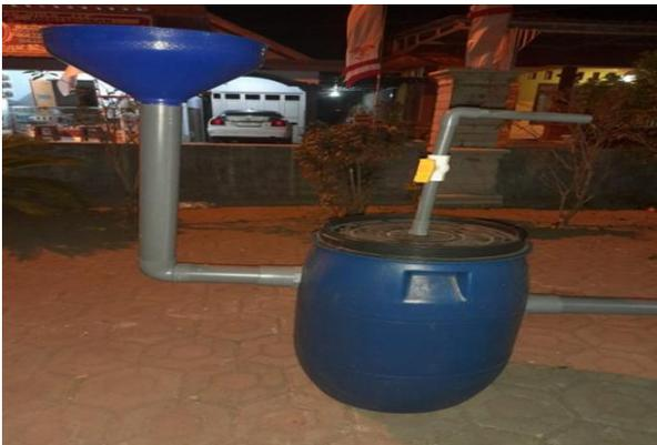
**Gambar 3** Prototype Digester Portabel
